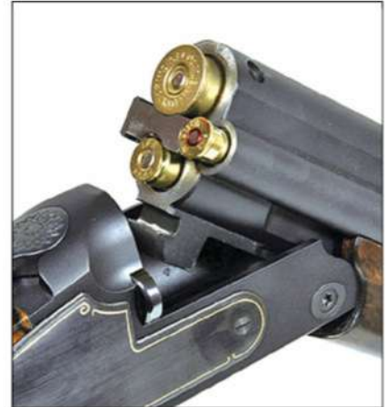
When “broken” open all three barrels of the Drilling could be loaded.
