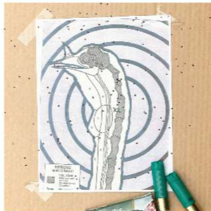
The second choke provided a much tighter pattern, with plenty of pellets in the kill zone.
