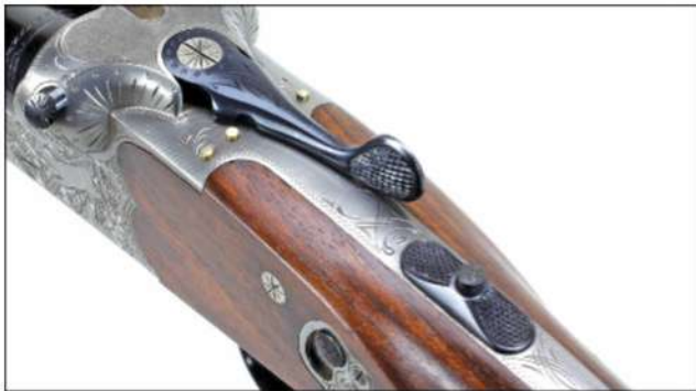
This close up of the Colt's receiver shows the safety, barrel selector switch and three cocking indicator buttons. (Rock Island Auction Co.)
