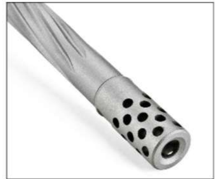
The barrel is cold hammer forged and features spiral fluting to reduce weight and a radial muzzle brake to reduce recoil. (Photo by Michael Anschuetz)
