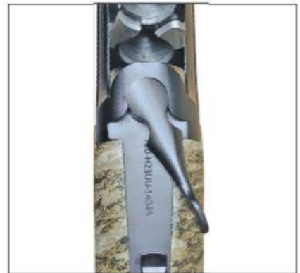
The tang safety is a standard affair. Left for the top-first shot, and bottom for right first.
